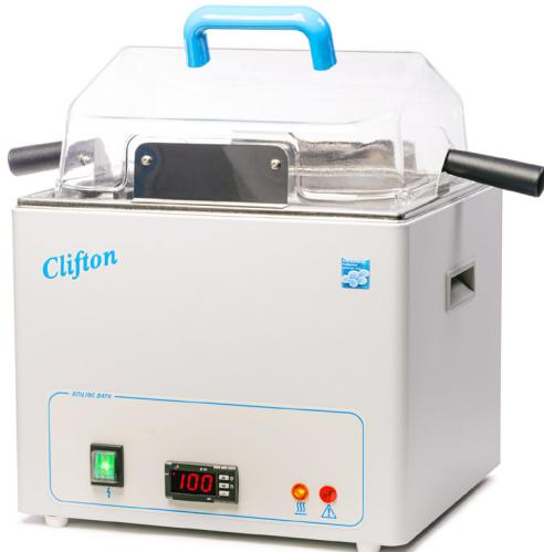
This range of boiling baths has been enhanced to include drain tap and clear lift off lid. Designed for applications that require continuous boiling. This bath also has the flexibility where the control can be regulated from a gentle simmer to a vigorous boil. Constant level device fitted on some models.
