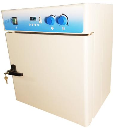
These digital scientific incubators can run at set temperature immediately, use run back timer or enable a delay start feature. Can be configured for gravity convection or with variable fan speed providing forced air circulation within the chamber.
